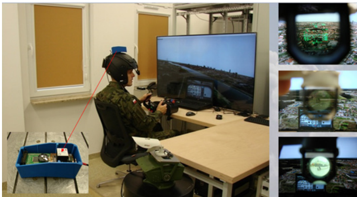
Figure 3. Laboratory test of ADIS16405 sensors in NSC-1 ORION system: a) deviation test stand of the helmet sensor (ADIS-16405_PO) and the reference sensor (ADIS-16405_SP), b) functional tests
