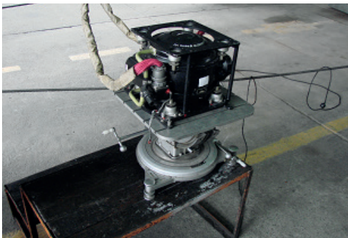
Fig. 10. View of the IKW-8 inertial navigation system on stand KPA-5 Source: P. Rogala, Statyczna Metoda Oceny... , op. cit.
