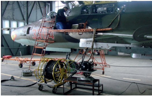
Fig. 1. View of Su-22 aircraft during IKW-8 system diagnostics in military unit conditions
