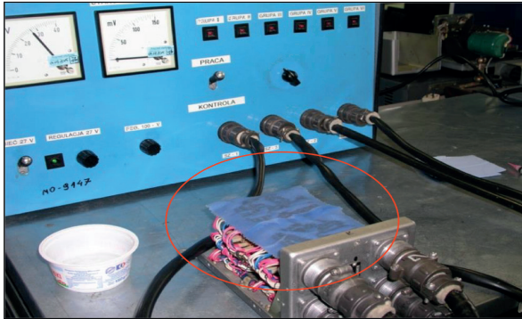
Fig. 12. Station for testing the SSP-FK-BI block in conditions of moisture (water) exposure Source: own elaboration.
