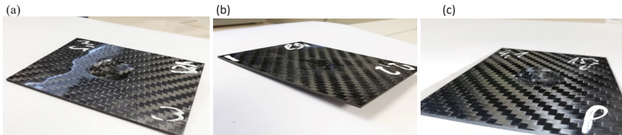
Fig. 6. Visual assessment of damage to samples loaded with 15 J, (a) vacuum bag method, (b) infusion method, (c) method of fabrication using a press hydraulic
