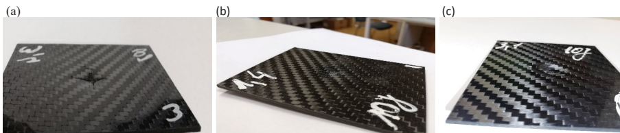
Fig. 5. Visual assessment of damage to samples loaded with 10 J, (a) vacuum bag method, (b) infusion method, (c) method of fabrication using a press
